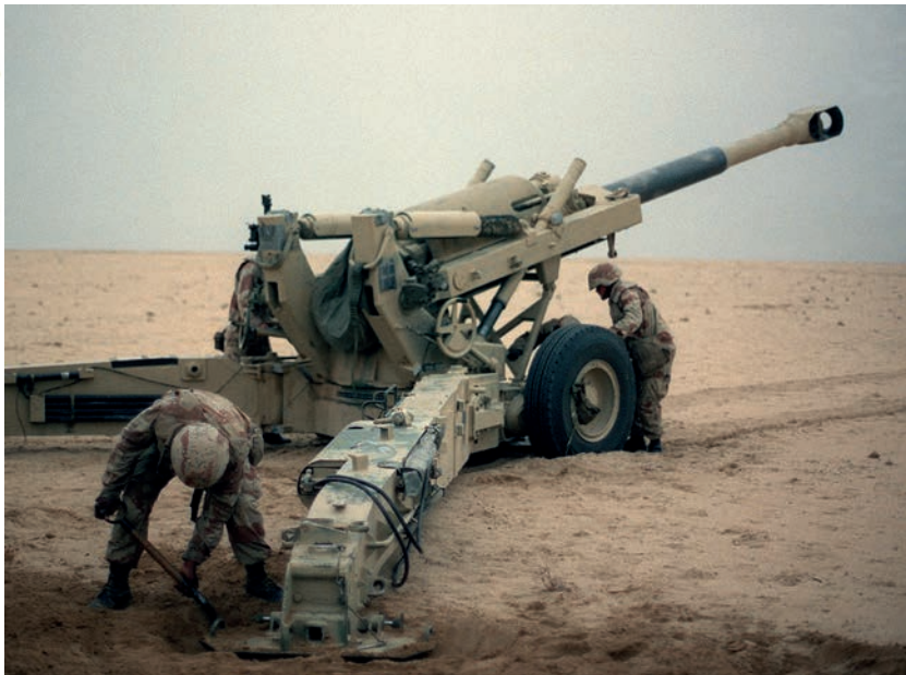
U.S. Marines during Operation Desert Storm set up an M198 155mm howitzer against Iraqi forces. Weighing more than 15,000 pounds, the heavy weapon had a reach of 14–18 miles.
